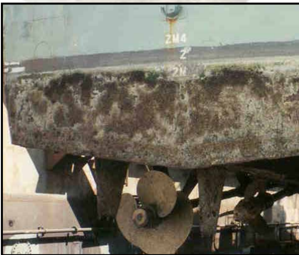
Figure 1 Fouling on hull of Royal Australian Navy (RAN) vessel (Photo courtesy of John Lewis)
